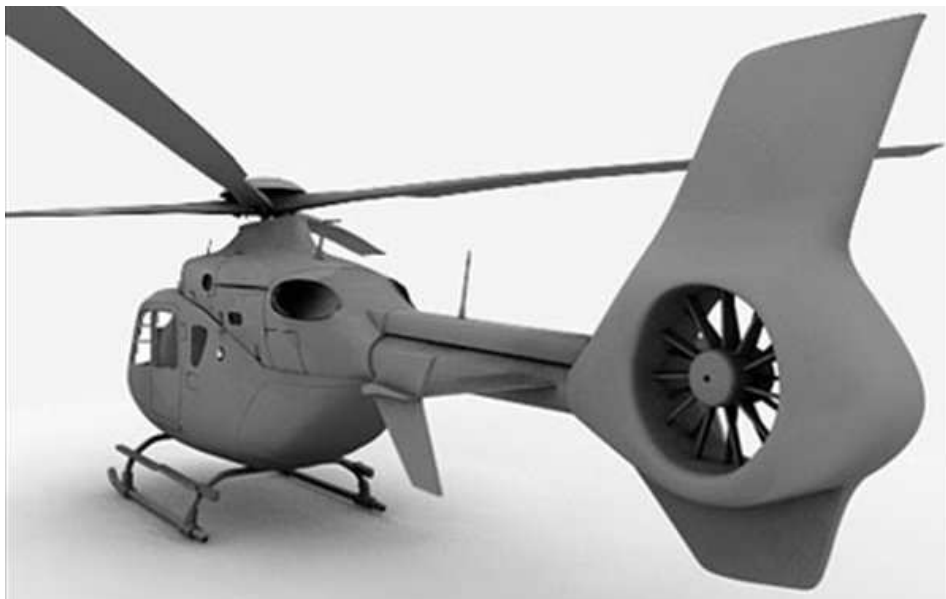
Slika 5.2. Helicopter Eurocopter EC 120 Colibri s repnim rotorom tipa fan-in-fin (ili fenestron)
